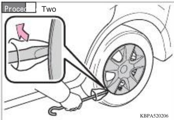
Di- ~Ya ~Tsu Key Ha Application De Le The Use For And, (e) Wheel cap \* Remove the.
