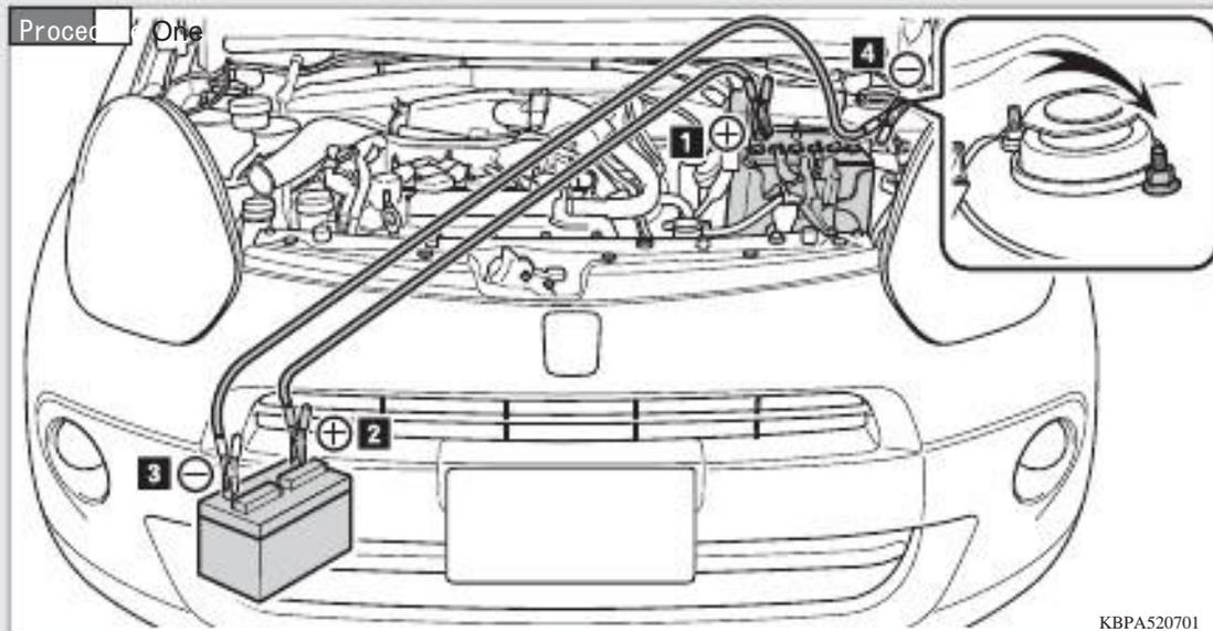
Of battery + Remove the terminal cover, the following order: the booster cable Connect with.
