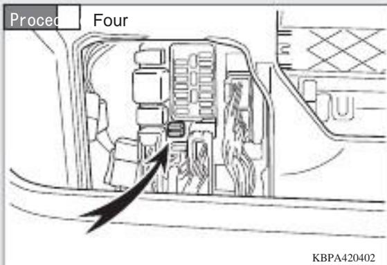
Pull the fuse in the fuse disconnect Pull the tree.
