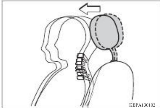
By the impact of the collision, the occupant's head is pushed forward a little bit. This will contribute to reducing injury.
