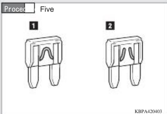
Check whether the fuse has not blown To.
